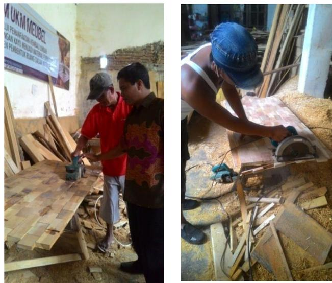
**Figure 2. Table Making Process of Wood Cut Waste**
